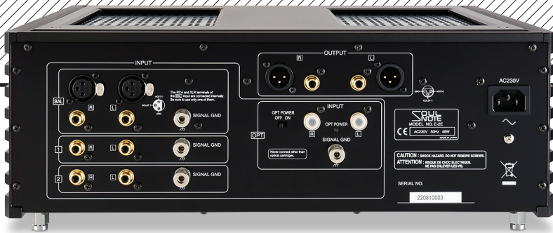
ABOVE: Up to three MM/MC pick-ups may be connected via RCA inputs (one on either XLR or RCA) with a DS Audio 'optical' cartridge hooked-up on adjacent RCAs (facilitating PSU out / signal return). Outputs are on RCAs and balanced XLRs
